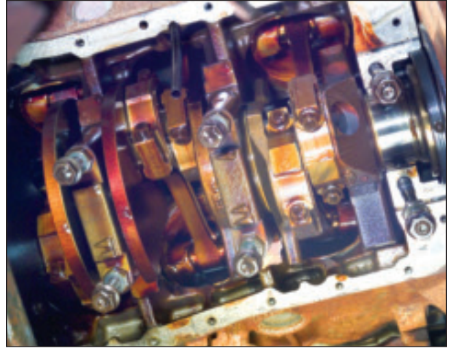
The lower crankcase area was very clean and free of any sludge deposits. The rear main bearing journal was removed showing no signs of visible wear on the crankshaft journal.
