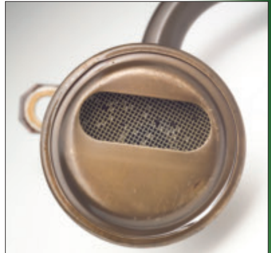
The oil pickup tube was very clean. There were minimal carbon deposits in the pickup tube screen..
